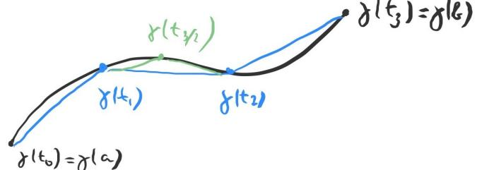
length relative to partition  $\tilde{\mathcal{T}}: \underline{\Lambda}(\tilde{\mathcal{T}}, \gamma) = \sum_{i=1}^n \|\gamma(t_i) - \gamma(t_{i-1})\|$
