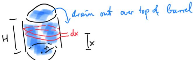
Work required to lift red layer over the top is the change in potential energy:
