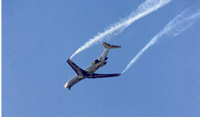
Fig. 4. This picture shows the wing-tip vortices which are associated with the circulation generating lift coming off the wings of a Boeing 727 aircraft. They were made visible by smoke generators installed on the tips of the aircraft wings. (NASA photograph number ECN-3831.)
